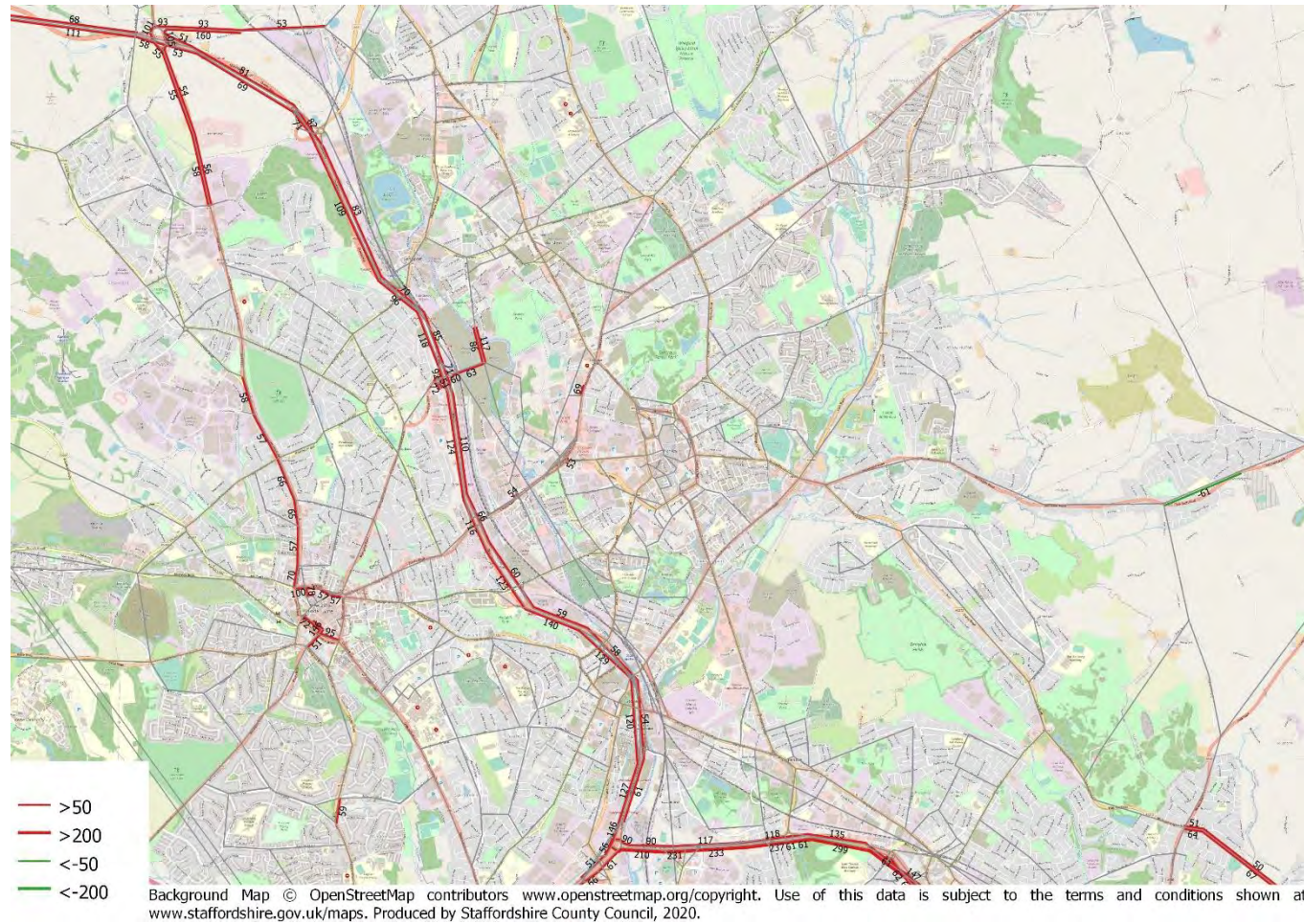
Figure 6-13: Change in Inter-Peak Hour traffic flows between 2022 Reference and 2025 Reference Case (vehicles)
